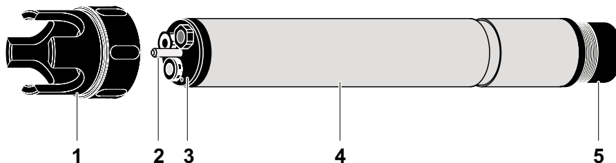
Fig. 1-2 Structure of the nitrate sensor NitraLyt ®Plus 700 IQ
