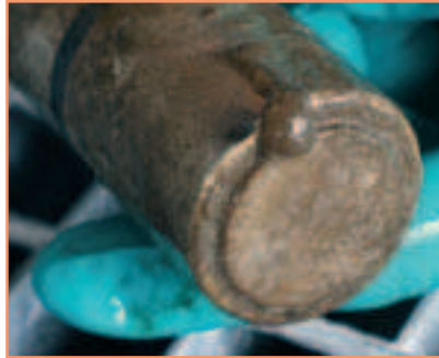
Sensor without ultrasound cleaning system After 16 Days
