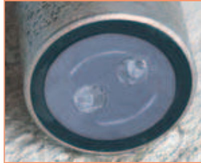
Sensor with ultrasound cleaning system After 16 Days
